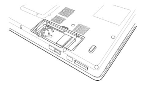
Figure 4- 10 Removing screws and disconnecting wireless LAN antennas
